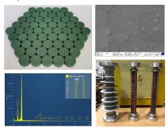
✓ Development of MOV discs based on (i) ZnO doped with V<sub>2</sub>O<sub>5</sub>, Sb<sub>2</sub>O<sub>3</sub>, Co<sub>3</sub>O<sub>4</sub>, SnO<sub>2</sub>, and Cr<sub>2</sub>O<sub>3</sub> (at TRL 7), and (ii) SnO<sub>2</sub> doped with Bi<sub>2</sub>O<sub>3</sub>, CuO, NiO, MnO<sub>2</sub>, ZrO<sub>2</sub> or Co<sub>3</sub>O<sub>4</sub> (at TRL 5) for MV surge arresters.
